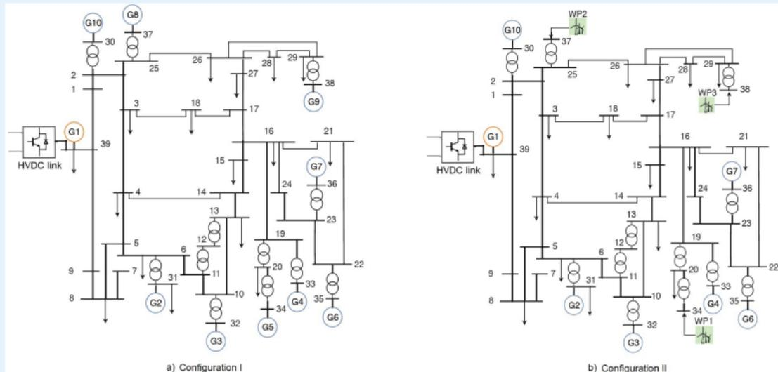
Test case: adaptive control of HVDC links for frequency stability enhancement
