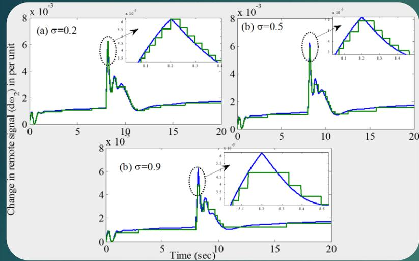
Comparison of remote signal in continuous and discrete mode for different sigma's
