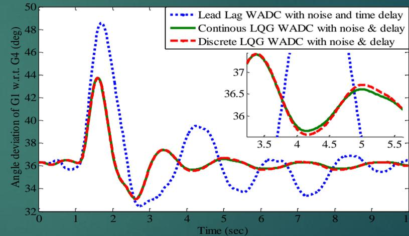
Fig. 4: With and without LQG controller, having time delay of 0.25 s and noise in remote signal
