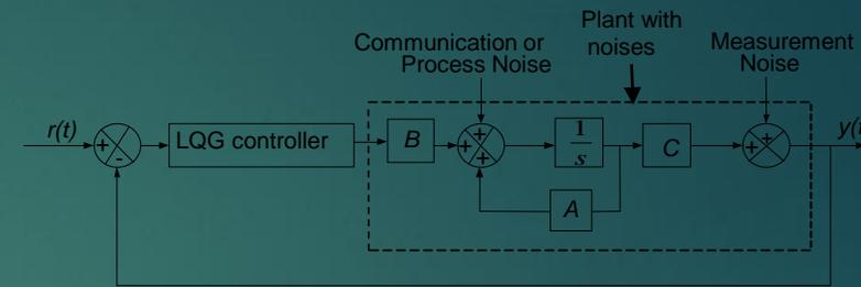
Fig. 2: LQG controller with Plant details
