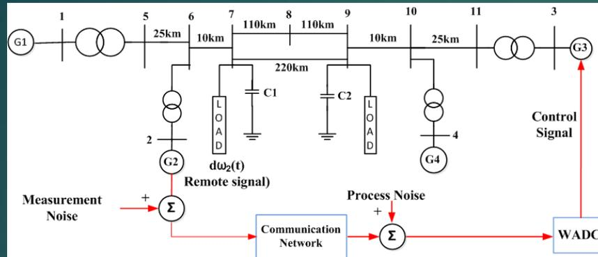
Fig. 1: Noisy test power system with WADC
