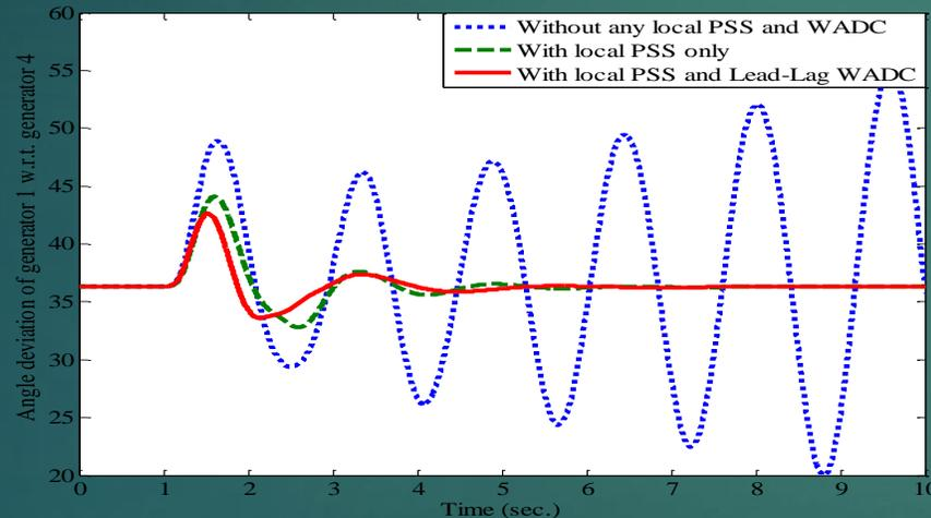
Fig.3: With and without lead-lag WADC, perfect medium
