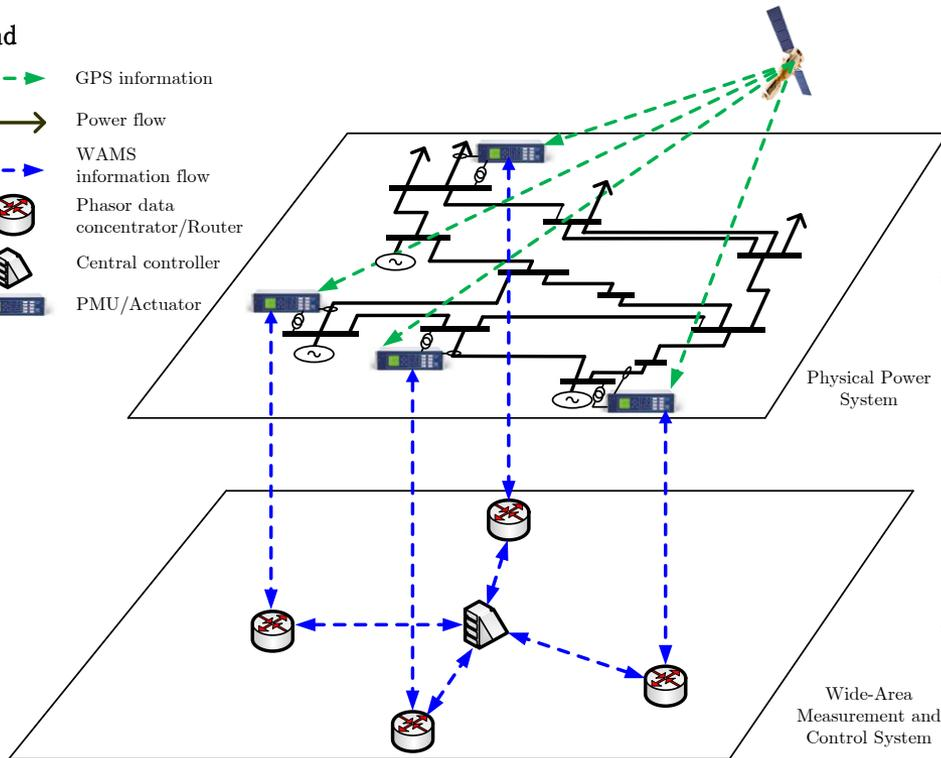
An illustrative diagram of the delayed cyber-physical power system (DCPPS)
