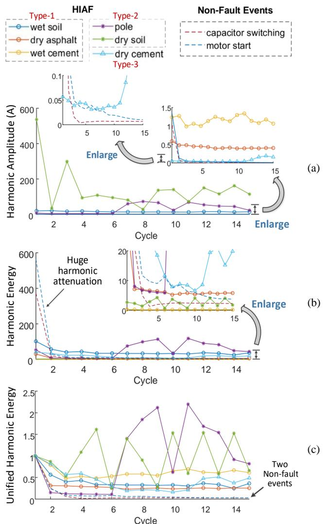
Non-fault events can be easier distinguished if using the unified harmonic energy for their dramatic harmonic attenuation.
