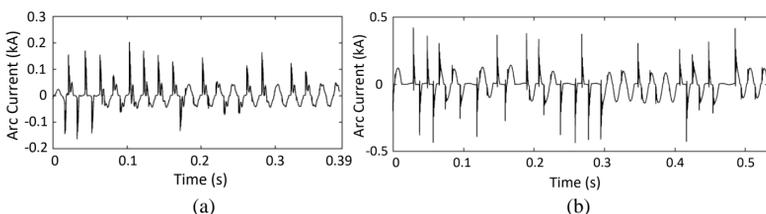
Comparison between the field (a) and simulated (b) waveforms
