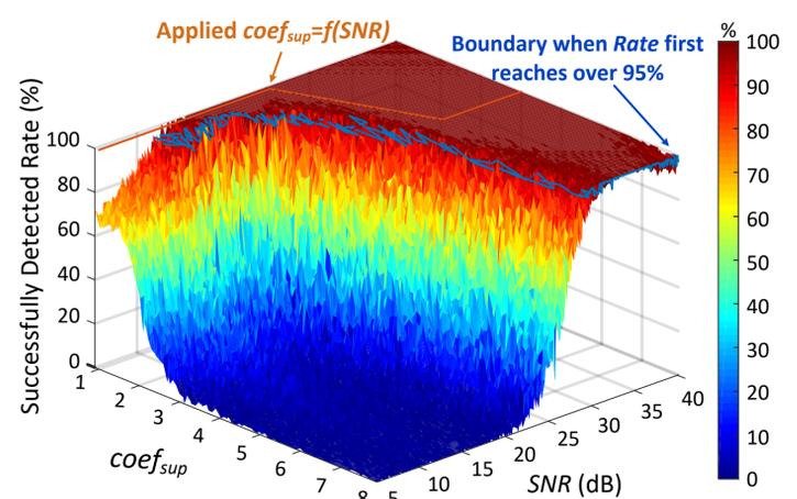
369 simulated Type-1 HIAFs with  $R_T$  from  $1\Omega$  to  $3k\Omega$ , which are all assumed with stable arcing periods.
