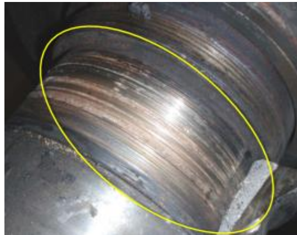
Bearing Inner Race Failure
