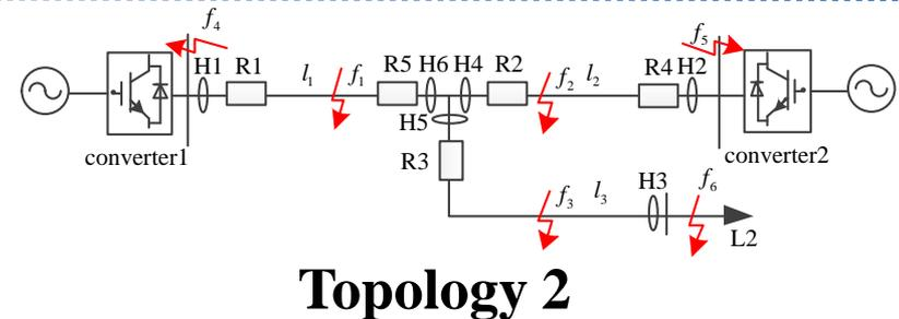
**Conclusion: Relay are located at the power side, and the MRs are located at the boundary point of the protection zone.**
