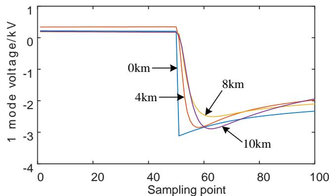
Different fault distance measured at R1
