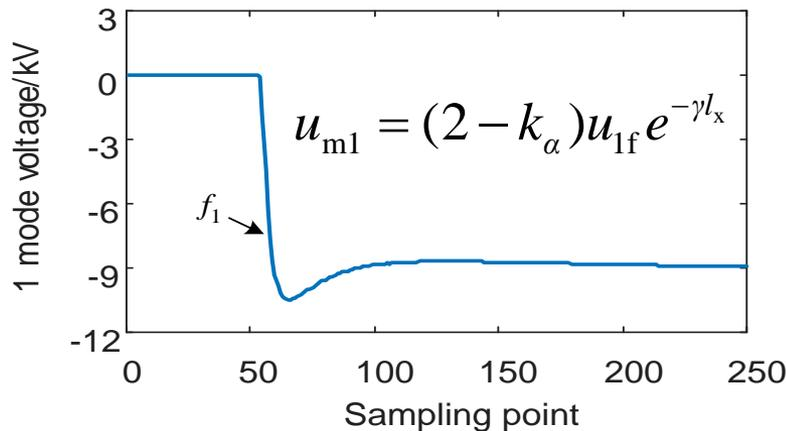
MRs can change the **steepness and peak time** of voltage of travelling wave in different fault points.
