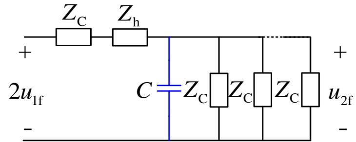
Refraction of voltage travelling wave
