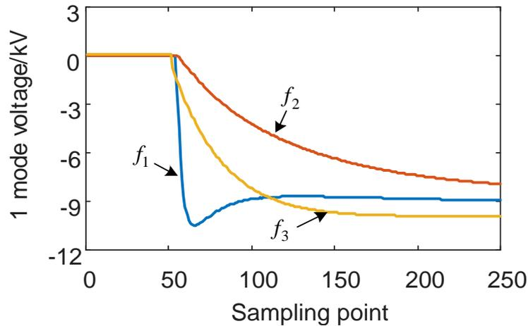
The threshold has to be smaller than the minimum peak time of forward external fault and reverse external fault
